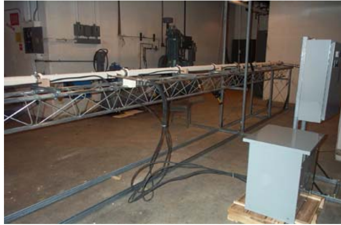
Figure 1. The state-of-the-art apparatus for lining 40-ft.-long heat exchanger tubes using impedance heating system
