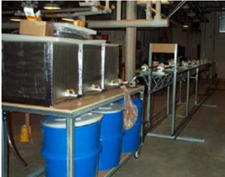
Figure 1. The state-of-the-art apparatus for lining 40-ft.-long heat exchanger tubes using impedance heating system
