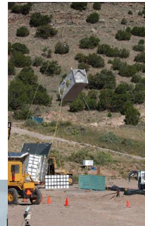
Full-scale drop test of TRUPACT III
