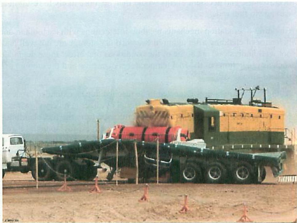
Figure 5. Spent-Fuel Crash Test
