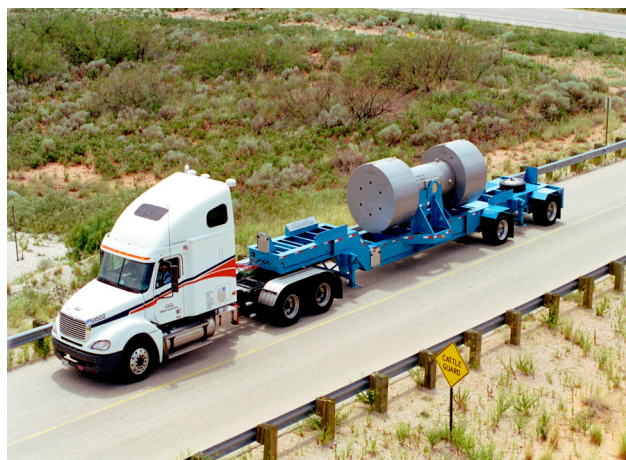
Fig. 6. Remote Handled nuclear waste (>100 nanoCi/gram of waste but <23 Ci/liter), some of it from reprocessing, being transported to the WIPP site in New Mexico in a 72B cask.
