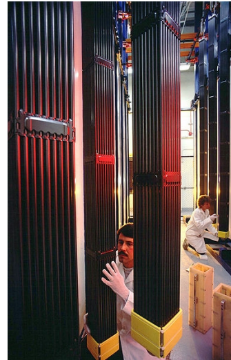
Figure 6. Workers Handling Fresh Nuclear Fuel Assemblies 19
