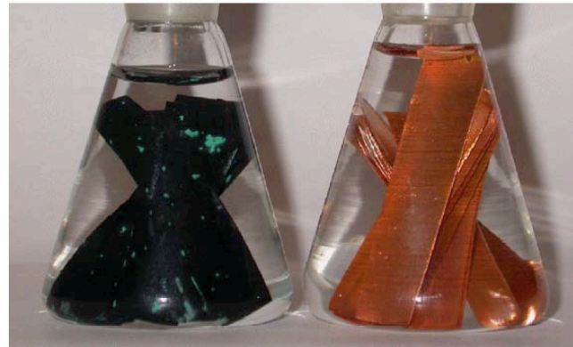
FIGURE 1 – Appearance of copper after 15 years of exposure in distilled water at room-temperature. Hydrogen from corrosion can escape from the left container but not from the container to the right. The water volume was equal in the flasks in beginning of the exposure.
