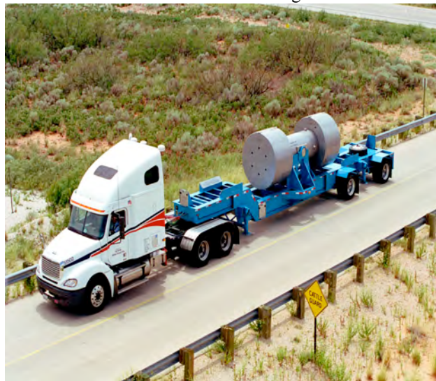
Fig. 4. High-activity remote handled nuclear waste, some of it from reprocessing of spent fuel from old weapons reactors, being transported to the WIPP site in New Mexico in a 72B casket. 10,000 shipments of nuclear waste to WIPP has never resulted in any release or harm to humans or the environment.
