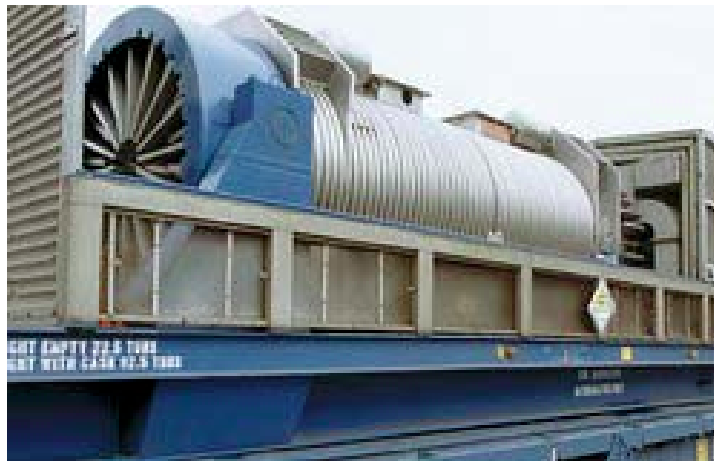
Figure 3-1 Typical Spent Nuclear Fuel Shipping Cask Mounted on a Railroad Car
