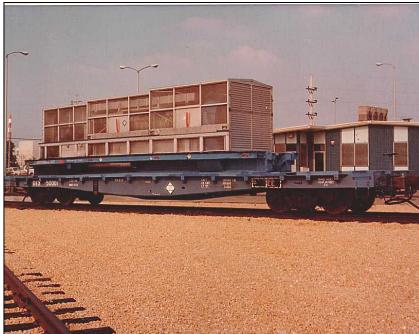
Figure 1-6 Rail Cask and Personnel Barrier Loaded on a Rail Car
