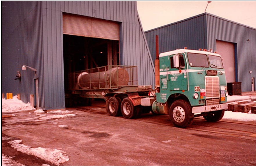
Figure 1-5 Truck Cask Ready for Transport
