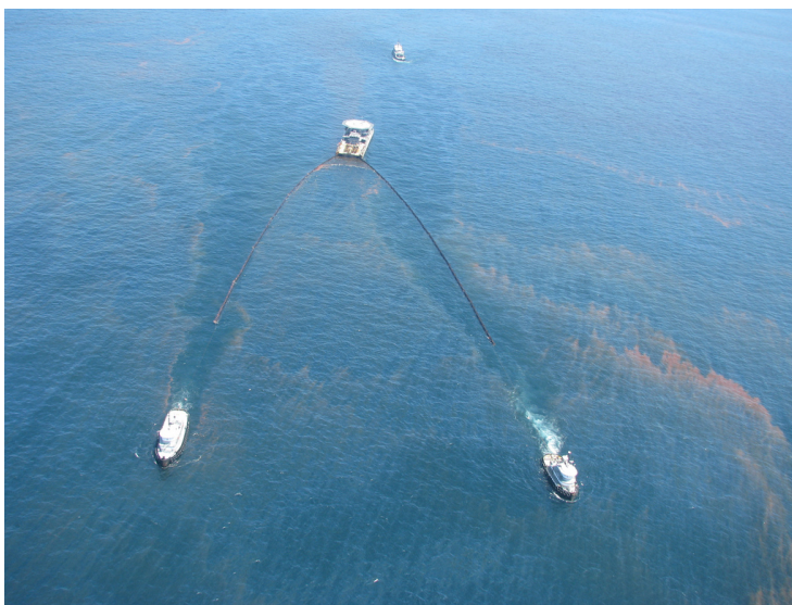
Towing boom to collect oil.
