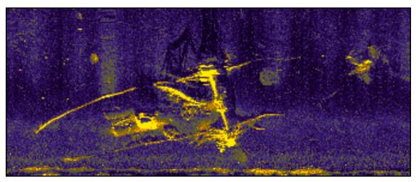
Figure B. Sidescan-sonar image of the Josephine.
