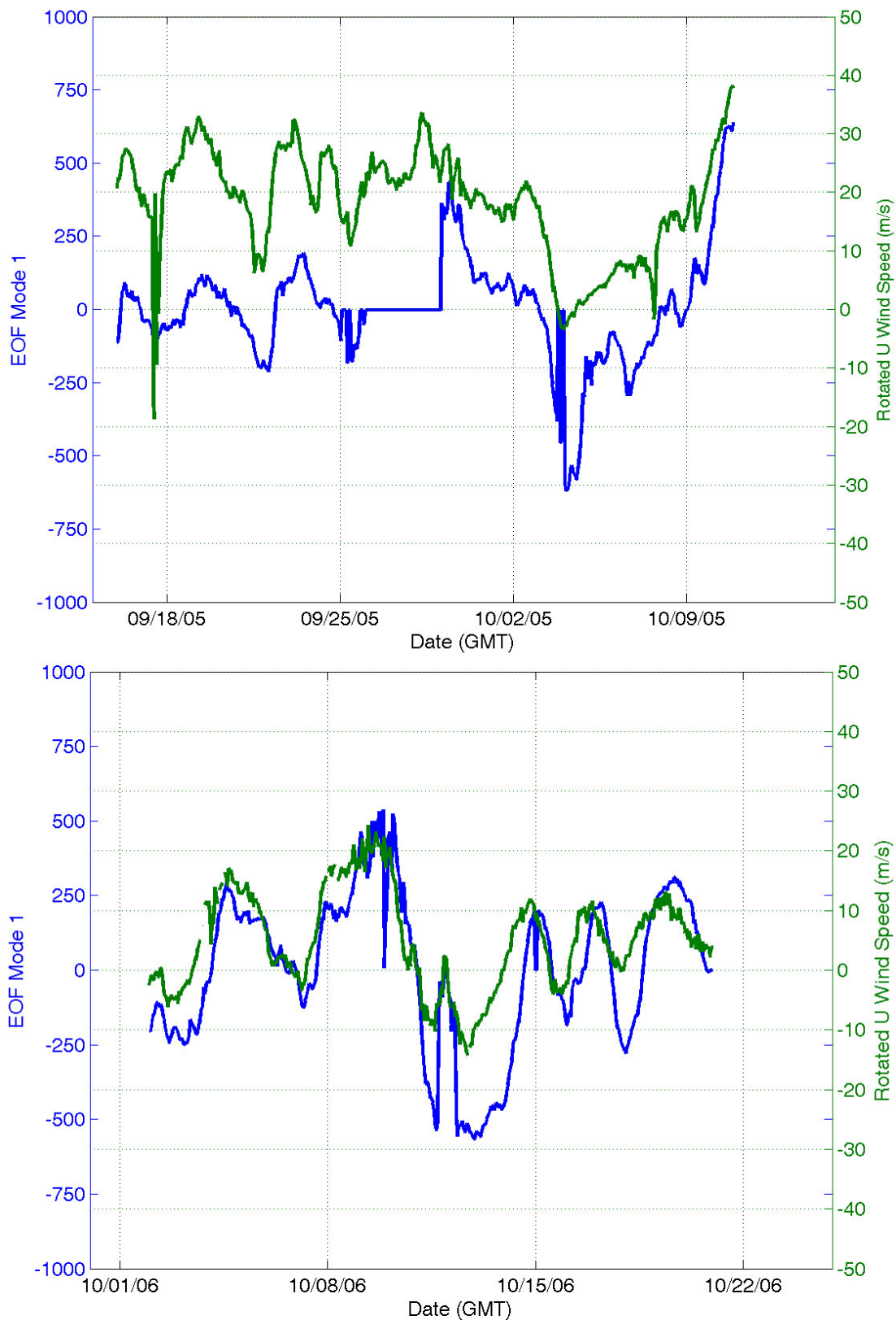
Figure 53. Time series of EOF mode 1 and wind speed from September 16 – October 10, 2005 (top), and October 2 – 20, 2006 (bottom).
