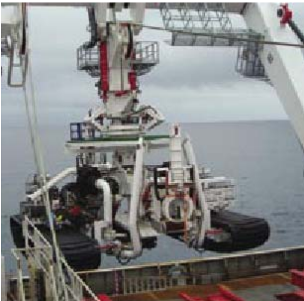
Figure 61 : Subsea cable burial devices [Ref. 7.7].
