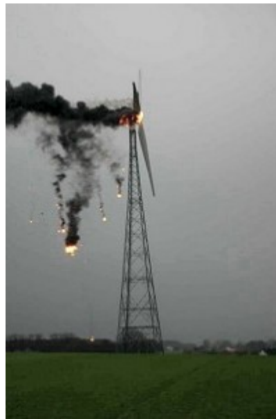
Figure 26: Examples of Lightning Damage [Ref. 3.7.8]
