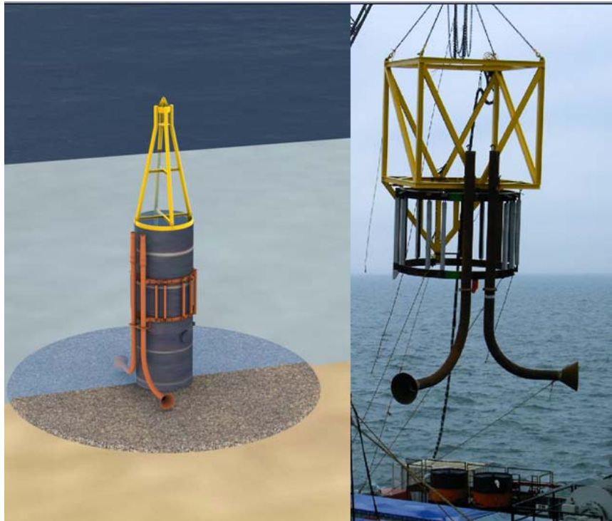
Figure 56: Arrangement of J-Tubes [Ref. 7.9].
