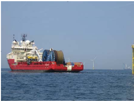
Figures 64: Cable laying vessel and cable deployment equipment [Ref. 7.9].
