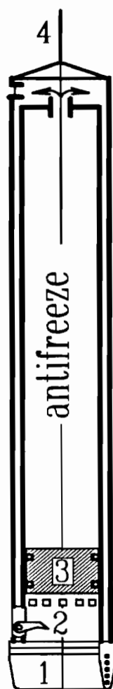
Figure 3. Antifreeze Thermal Electric Drill (ATED): 1 -drilling head; 2- core catchers; 3 - piston; 4 - cable.
