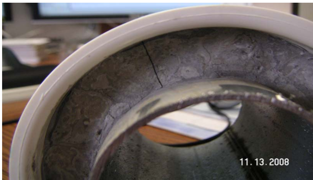
Fig 4.50: Cracks in 3-½" ID Pipe with 16 lb/gal Slurry after 30 Cycles
