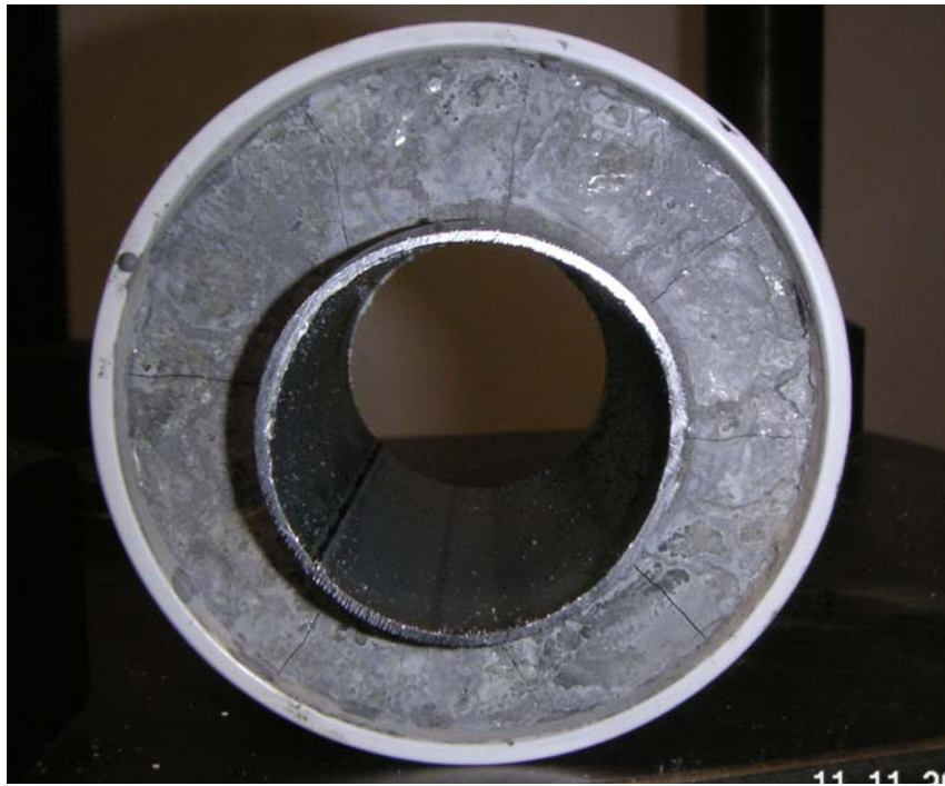
Fig 4.48: Cracks in 4-½” ID Pipe with 16 lb/gal Slurry after 30 Cycles
