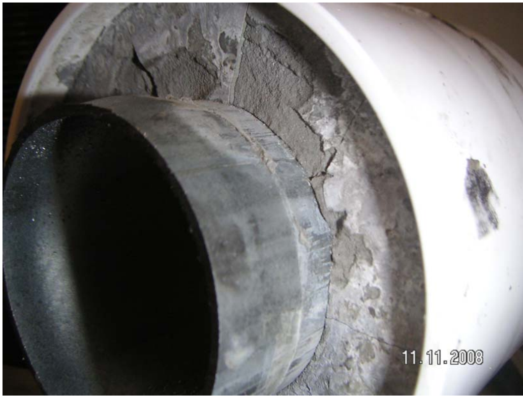
Fig 4.51: 4-½" ID Pipe with 16 lb/gal Slurry after De-bonding at 2,500 lb Force
