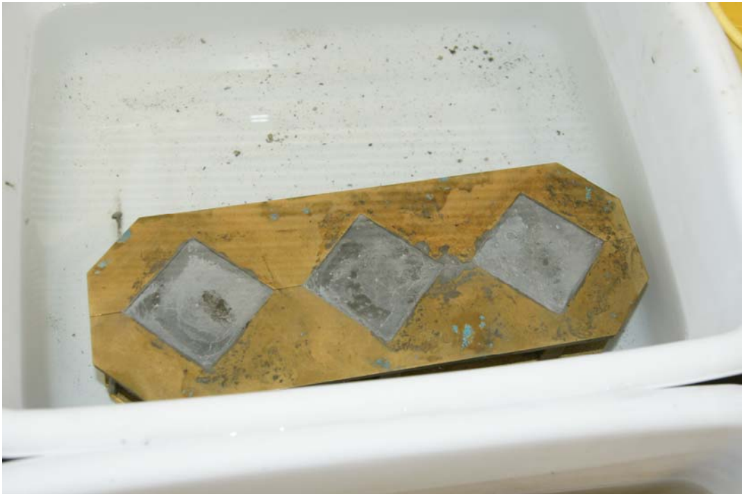
Fig 4.44: Cubes Cured Under Water at Atmospheric Pressure
