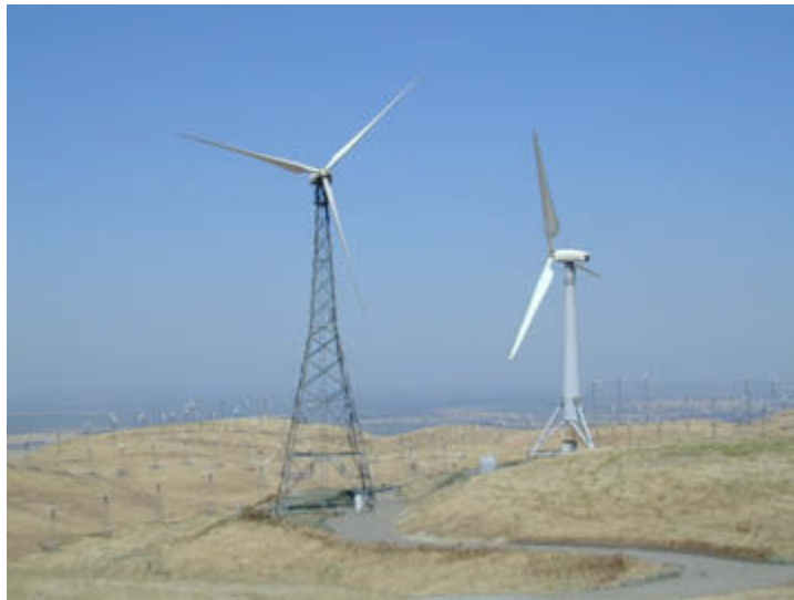
Photo 1-5. KVS-33 turbines on lattice and tubular towers in the foreground, and KCS-56 100-kW turbines in the background, view northeast.
