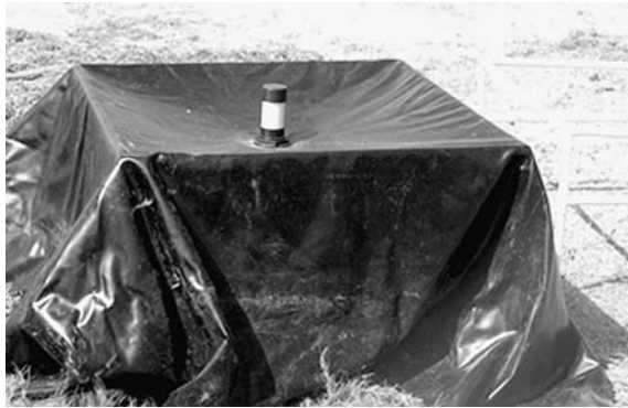
Figure 3. Underwater containment and treatment system used to apply chlorine (liquid sodium hypochlorite) to colonies of C. taxifolia in Agua Hedionda Lagoon. 20 mil black PVC covers PVC frame. Fitting at top is port through which liquid sodium hypochlorite was pumped by scuba divers (photograph by L. Anderson).
