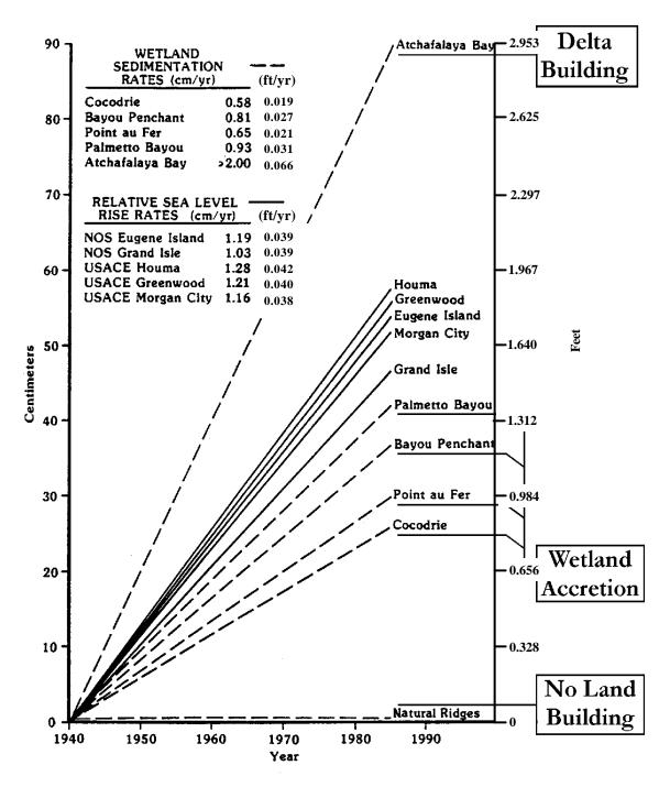
Figure 85. Comparison of RSL rise rates and wetland sedimentation rates for the Terrebonne Deltaic Plain area. Only in the Atchafalaya River Delta was land building up at rates higher than RSL rise. Wetland sedimentation rates are from DuLaune et al. (1985), and RSL rise rates are based on records from USACE and NGS tide gauges (adapted from Penland et al. 1988).
