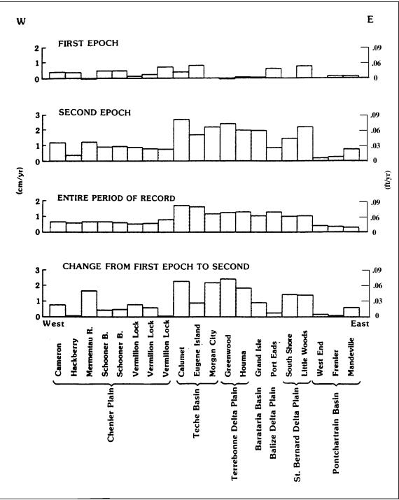
Figure 71. Relative sea level rise based on readings from U.S. Army Corps of Engineers tide gauge stations on Louisiana. Note change in rate of rise between 1947-1961 (Epoch 1) and 1962-1978 (Epoch 2) (after Penland et al. 1989).
