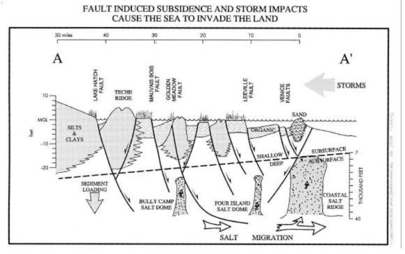
Figure 67 Cross-section through the Terrebonne Deltaic Plain after modification by fault and storm events. During the deterioration stages of the cycle fault events reduce the land surface and facilitate invasion of the land by the gulf. Reduction of land elevations in reference to the gulf level is largely due to deep-seated salt and fault movement.
