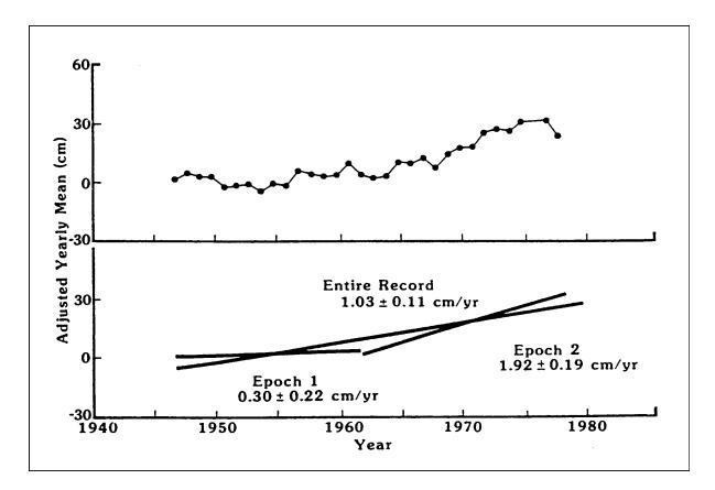
Figure 70. Water level time series from National Ocean Survey, Grand Isle, LA. Tide gauge between 1947 and 1978. A change in the rate of rise between the period 1947-1962 (Epoch 1), and the period 1962-1978 (Epoch 2) had been found on many of the records from gauges in south Louisiana (after Penland et al. 1989:24).
