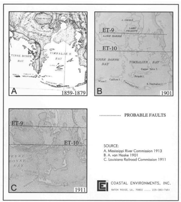
Figure 56. Comparison of historic maps showing the severance of the natural levees of Bayou Terrebonne and the opening of Lake Barré between 1859-1879 and 1901. The locations of suspect faults have been added to the maps.
