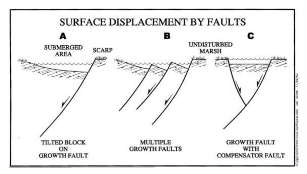
Figure 18. Common types of faults found in the study area showing linkage between surface features and underlying fault planes. Based on surface and subsurface data.
