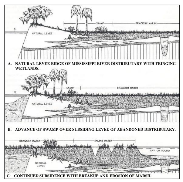
Figure 90. Effects of subsidence on natural levees and wetlands (modified from H.N. Fisk 1960).
