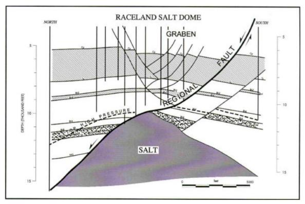
Figure 10. Cross-section of the Raceland Salt Dome, which lies within the Lake Salvador Fault Zone (after P.J. Pickford et al. n.d.). Note the counter-basinward fault, the crestal graben with nested faults and the top of the high pressure zone.
