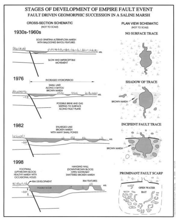
Figure 89. Stages of fault event in a saline marsh.
