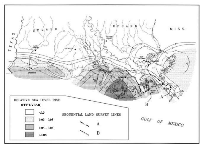
Figure 74. Isopleth map of RSL rise rates in coastal Louisiana based on 1962-1982 (Epoch 2) tide gauge data (adapted from Ramsey and Moslow 1987). Locations of sequential land leveling lines are also shown.
