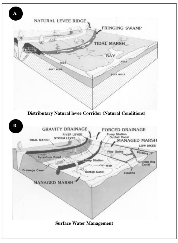
Figure 91. Effects of subsidence on ridgelands and fastlands. A. Distributary natural levee corridor, natural conditions. B. Subsided distributary natural levee corridor with forced drainage and storm protection levees (after Gagliano 1990).
