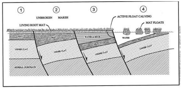
Figure 87. Diagrammatic section showing effects of fault movement on root mat and near-surface deposits.
