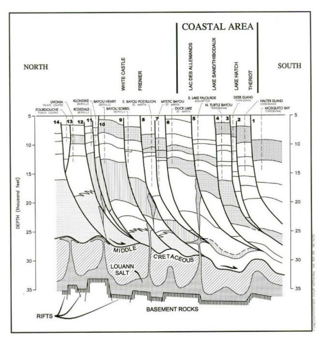
Figure 8. North-South cross-section through the Gulf Coast Salt Dome Basin showing stratigraphy and geological structures (after Adams 1997). Extensional section with progressively younger listric faults from north to south. Section also shows inferred basement-salt-decollement surface relationships. Subsurface faults shown in Figure 6 are identified on the section.
