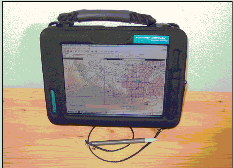
Figure 3—Pen tablet PCs have a simpler hardware profile compared to the laptop-based system.
