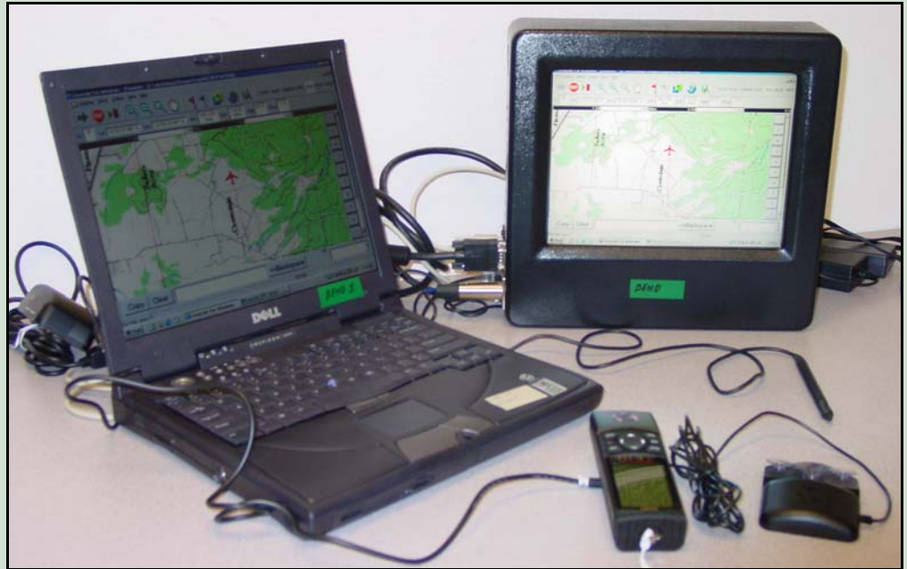
Figure 2—The majority of forest health aerial surveyors use this laptop PC-based system. The Dell 8000 PC, Garmin 12XL GPS Receiver, and KDS touchscreen are shown above.
