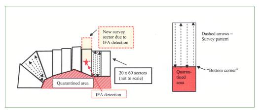
FIGURE 2-1: Survey Pattern for Large Block Design
