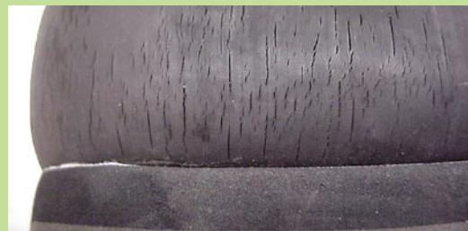
The toe of this rubber wader boot has cracked after being exposed to repeated applications of benzethonium chloride. (Photo by Robert Hosea.)
