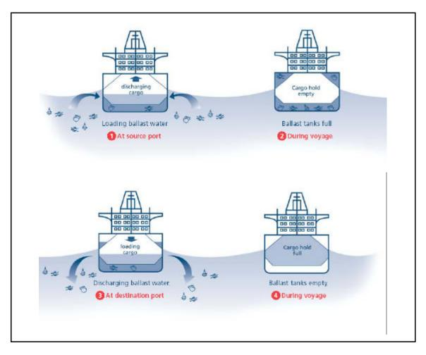
Figure Four: The ballast water cycle (Source: GloBallast Programme, IMO).
