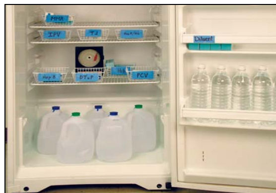
Water bottles as buffers in refrigerator to stabilize temperatures
