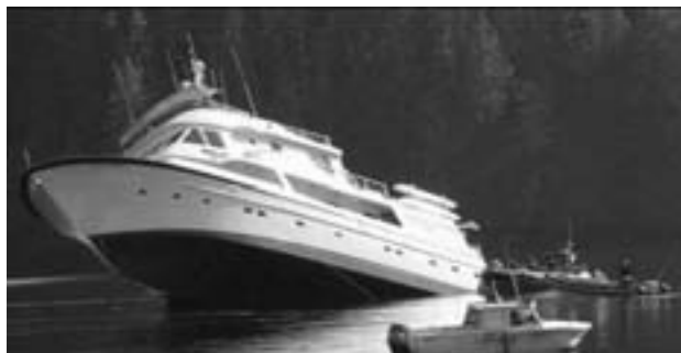
The Safari Spirit listing to starboard at an angle of about 35° when it shifted on the submerged rock. ( Photograph courtesy of Shearwood Marine.)
