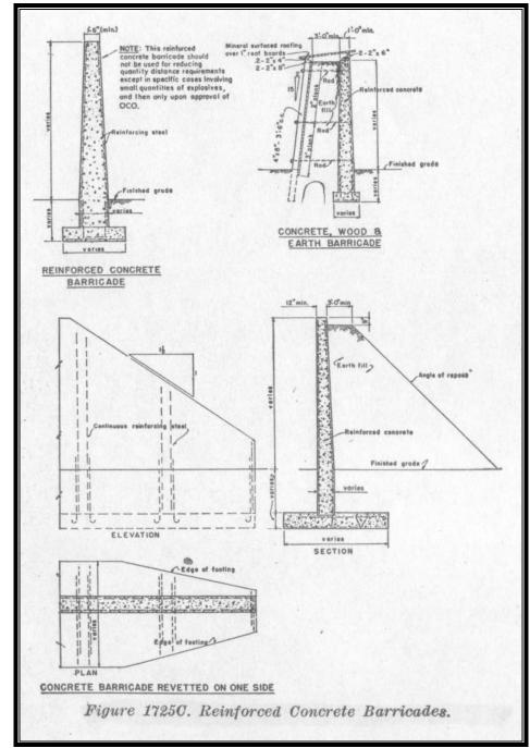
Plate 6.15 Plans of various concrete barricades (Ordnance Corps 1951:17-31)
