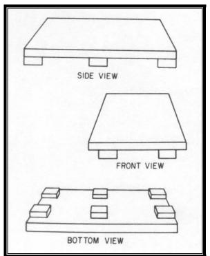
Plate 8.5 Pallets designed for four-sided lifting for efficient handling (Ordnance Corps 1961:136)
