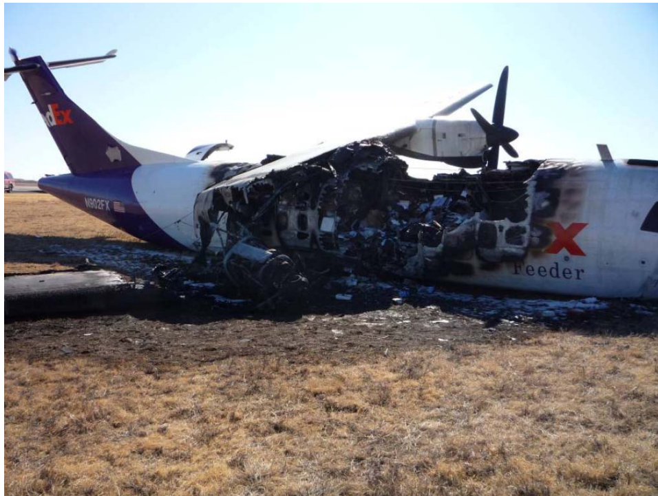
Figure 6. Right side of fuselage showing extensive fire damage to right wing and flap components.
