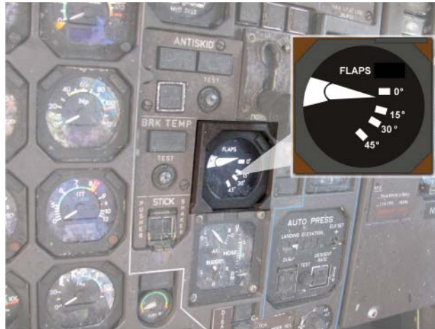
Figure 2. Flap position indicator. Inset shows the likely needle pointer position during the flap asymmetry.
