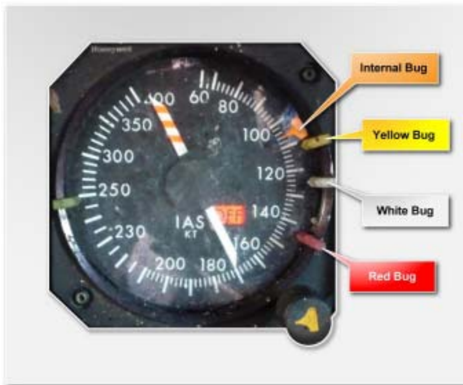
Figure 4. Airspeed indicator showing needle pointer; selector knob; and internal, yellow, white, and red bugs.
