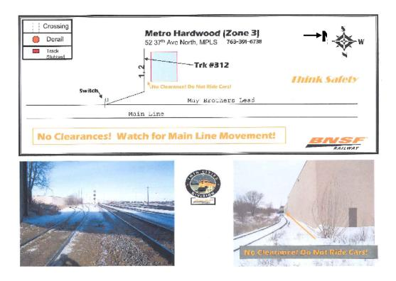
**Figure 2.** "No Clearance" warning for Metro Hardwoods in the BNSF *Northtown Terminal Spotting Profiles and Risk Identification Storybook*, which was in effect at the time of the accident.
