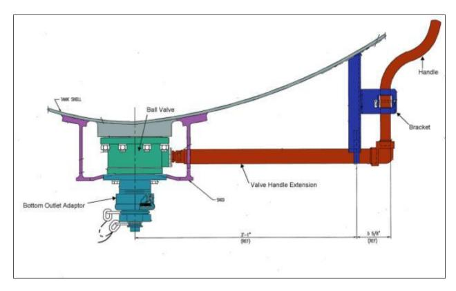
**Figure 8.** Bottom outlet valve arrangement (not to scale) used on derailed NATX and TILX tank cars. (Adapted from a Trinity Tank Car drawing)
