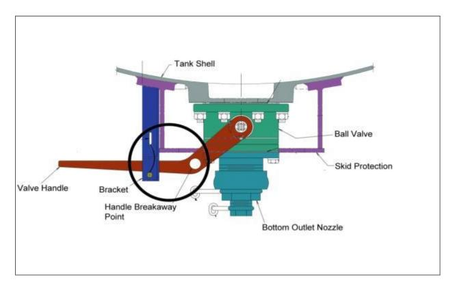
**Figure 7.** Bottom outlet valve configuration, as modified from original design, for derailed CITX and CTCX cars. (Not to scale) The operating handle securing bracket is circled. (Adapted from a Trinity Tank Car drawing)
