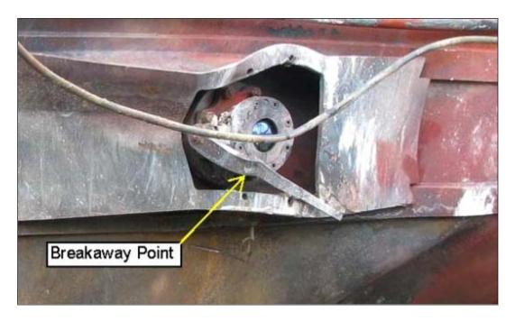
**Figure 11.** Bottom outlet valve of car CTCX 731599 showing exposed valve and bent but intact valve operating handle. Handle retaining bracket is missing. (Valve was opened during derailment but was closed by emergency responders.)
