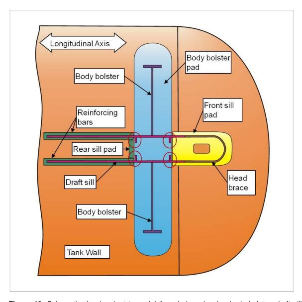
**Figure 19.** Schematic drawing (not to scale) from below showing body bolster, draft sill, and head brace attachment locations to pads on underside of tank cars. Circled areas indicate where transverse portions of draft sill are welded adjacent to transverse weld of body bolster pad.
