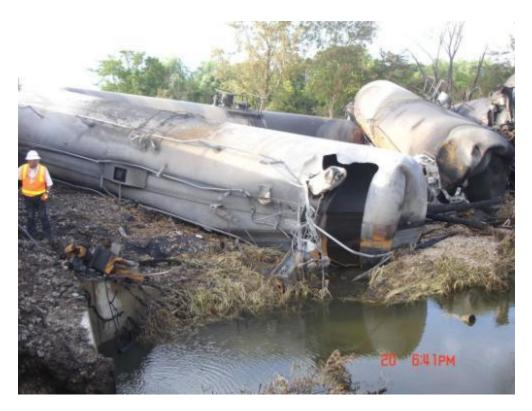
Figure 10. Breach in tank car NATX 303504. (Federal Railroad Administration photo)
