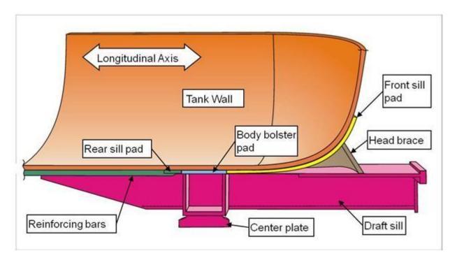
Figure 18. Schematic cutaway view (not to scale) of end of tank car showing major components.
