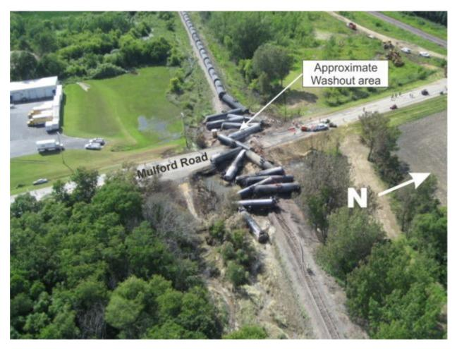
**Figure 3.** Aerial view, looking northwest, of derailed tank cars after locomotives and first 58 cars have been pulled away from wreckage.
