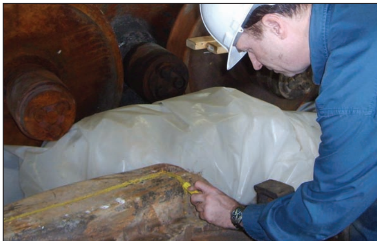
A railcar truck side frame sample is being marked for laboratory analysis of rail burn scars.
