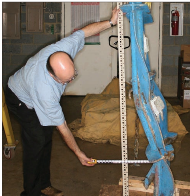
Evaluation of damage to the rudder from the fishing vessel Lady Mary
