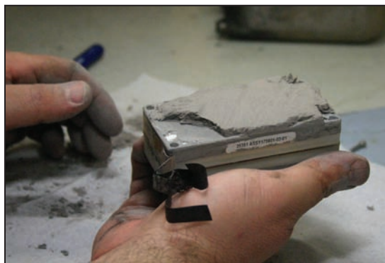
Vehicle Recorder Division staff extract the memory from a damaged solid-state combination CVR/FDR and prepare the memory to be downloaded using laboratory equipment.
