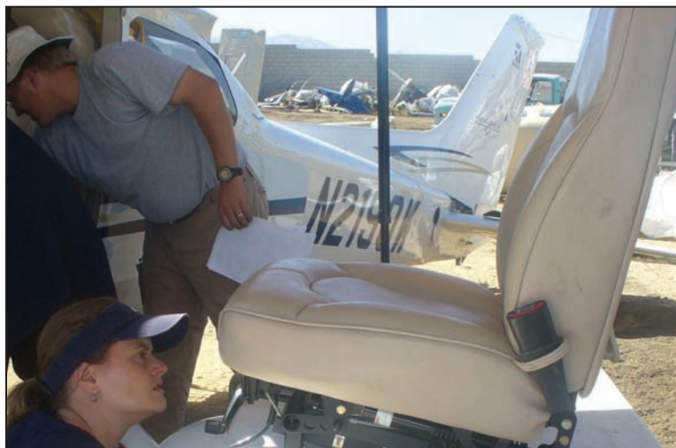
An NTSB biomechanics specialist documents seat damage for the GA airbag safety study. The accident, which occurred on September 30, 2008 in Fullerton, California, and involved an airbag-equipped Cessna 172S (LAX08FA301), is one of the cases being considered in the airbag study.
