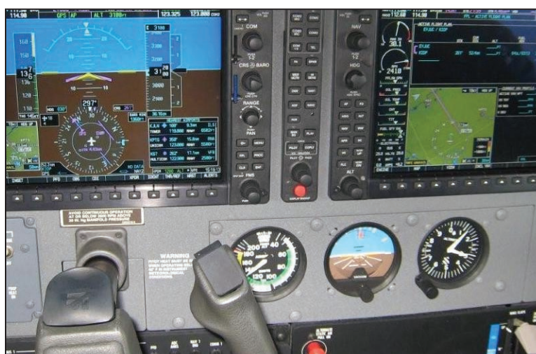
Example of a light aircraft glass cockpit.
