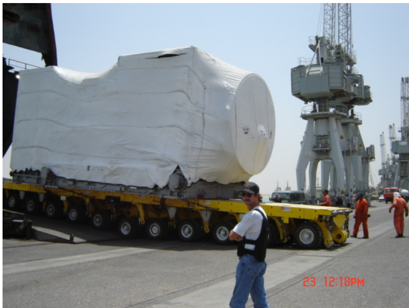
Photo 2. This photo, taken June 23, 2004, shows one of the two GE Frame 9E turbines off-loading from the ship at the Iraq port of Umm Qasr.
