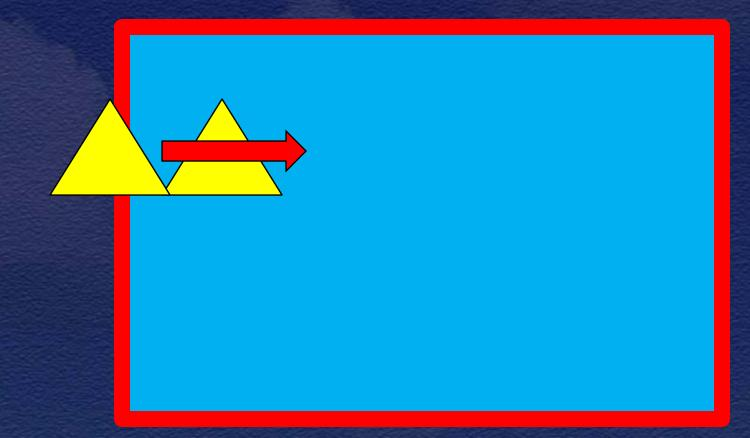
If the operator attempts to operate outside of "the box," the automation informs, cautions, or warns, the operator to return to within the box, or automatically takes over to place vehicle back within the box.
