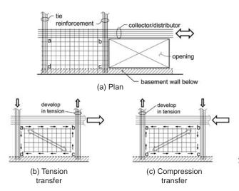
**Figure 7-3** – Reinforcement to transfer collector / distributor force around an opening.
