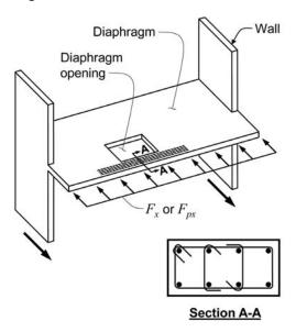
**Figure 7-1** – Confinement reinforcement in axial struts around openings.
