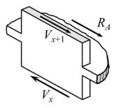
**Figure 5-1** – Force  $R_A$  transferred between diaphragm and wall can be obtained by section cuts through wall.
