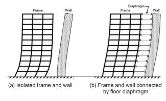
**Figure 4-3** – Diaphragms develop transfer forces by imposing displacement compatibility between different vertical elements of the seismic-force-resisting system.
