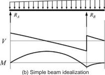
Figure 6-2 - Corrected equivalent beam model.
