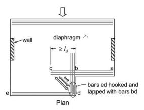
Figure 7-4 – Reinforcement associated with re-entrant corners.
