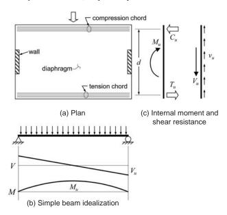
Figure 3-1 – Tension and compression chords.
