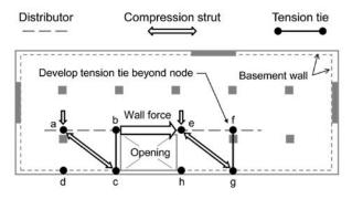
Figure 6-9 – Strut-and-tie model at force transfer to basement wall.
