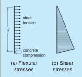
For the extreme case of uniformly distributed flexural steel, with all steel assumed at the yield stress, the shear stress increases linearly from zero at the edge to a maximum value of approximately  $2V_u/td$  at the neutral axis.
