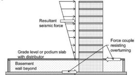
**Figure 6-3** – The force couple resisting overturning in walls at the podium level and below is known as the backstay effect.
