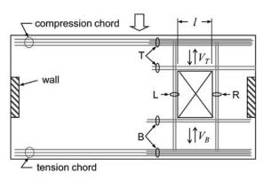
Figure 6-10 - Diaphragms with large openings.
