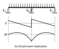
Figure 6-1 - Equivalent beam-on-springs model.
