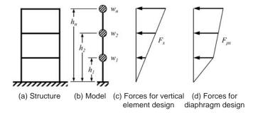
Figure 4-2 – Design forces for vertical elements and diaphragms.
