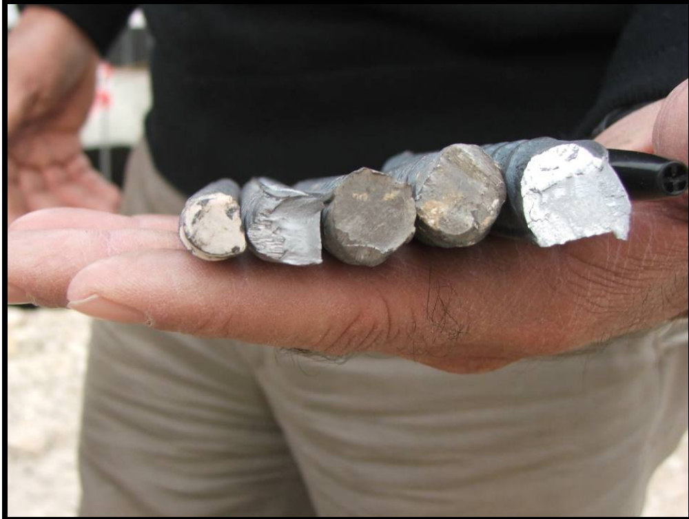
Site Photo 1. Rebar varied between .375" and .675" diameter depending on application.
