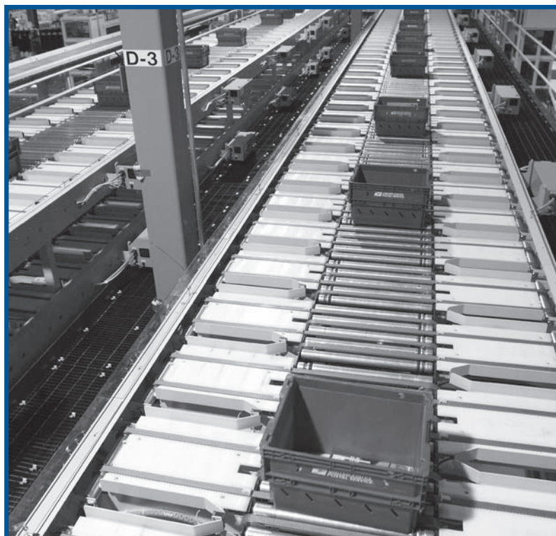
The Flats Sequencing System (FSS) is intended to boost efficiency in processing, distribution, and delivery. FSS automatically sorts flat-sized mail into delivery point sequence at high speeds. OIG audits analyze how delivery operations have improved as a result of receiving flat mail in walk sequence from the FSS.
