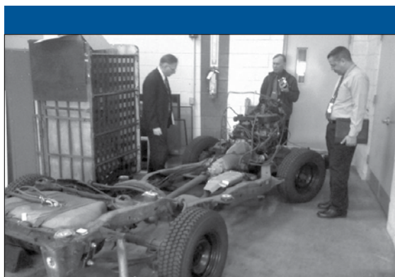
Postal Service vehicles are being completely reassembled to include frame, engine, transmission, and body shell. Available data shows 613 vehicle frames were replaced in FY 2008 and 2,250 frames in FY 2009.
