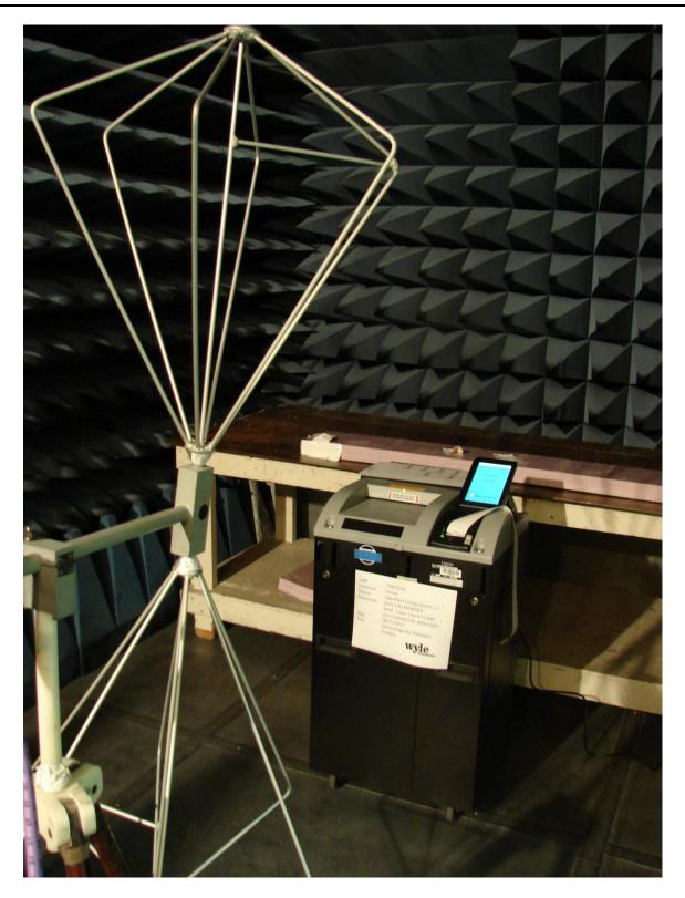
Photograph No. 14 Electromagnetic Radiation Analysis – 4
