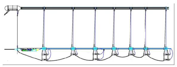
Figure 2. One linear airgun array or string with ten airguns, nine of which would be operating.
