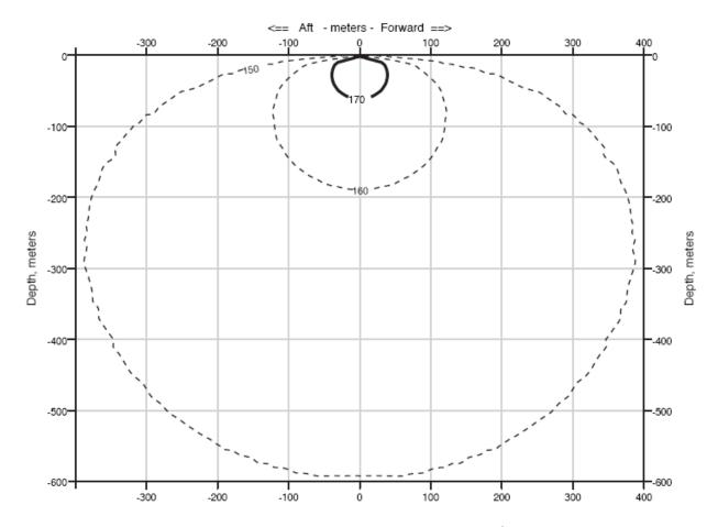
**Figure 3.** Modeled received sound levels (SELs) from a single  $40 \text{-in}^3$  airgun operating in deep water at a 9-m tow depth. Received rms levels (SPLs) are likely ~10 dB higher.
