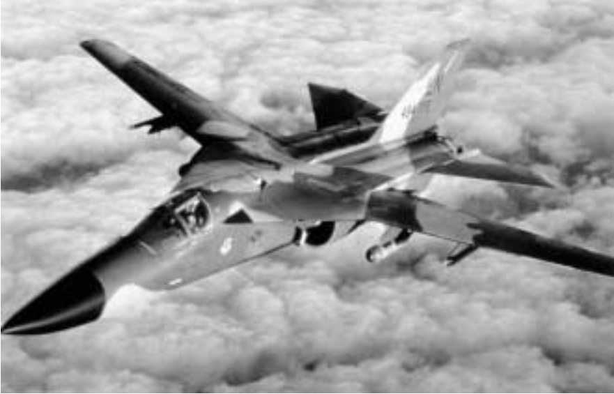
The F-111, sometimes called the Aardvark, featured swing wings that could be swept forward for slow flight or backward for greater speed.
