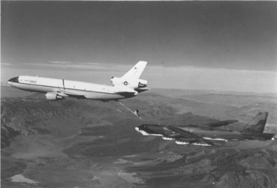
B-52 and KC-10. Although designed to deliver nuclear weapons, long-range bombers can add significant punch to theater conventional operations. Here, a B-52 bomber refuels from a KC-10 tanker.
