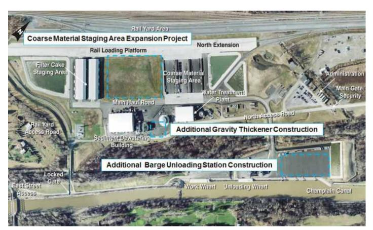
Figure 1: Processing Facility improvements for winter/spring 2012 include expansion of the coarse material staging area and construction of a second barge unloading station, additional size separation equipment, and a second gravity thickener.
