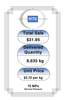
**Figure 1.** Examples of the Product Identity, Measurement Unit, Unit Price, and Service Pressure on the User's Interface of a Hydrogen Fuel Dispenser
