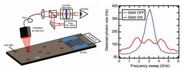
Figure 3.2: Left: Schematic diagram of apparatus used to "shake" a self-assembled quantum dot and resolve the fluorescence. Right: Fluorescence spectrum of quantum dot (blue curve) acquires resolved sidebands (red curve) when "shaken" by surface acoustic wave.
