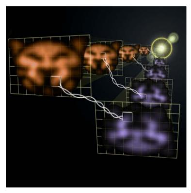
Figure 3.3: Composite of quantum-correlated images indicating approximate regions of quantum correlations between the "twin" images. The pair of images is created by sending a seed image through an atomic vapor cell in which the 4-wave mixing process amplifies the seed and also generates the twin image.
