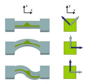
Figure 2.3: Pyramidal InAs quantum dots in a flat nanomechanical beam, a beam providing biaxial deformation and a beam under shear. The rotation of the polarization of the ground exciton (purple) and exchange-split exciton induced by the indicated mechanical strain is demonstrated.
