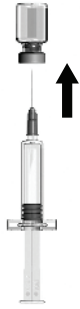
Figure 1. Cleanse vial stopper. Attach appropriate needle to accompanying prefilled syringe of saline diluent and insert into vial.
