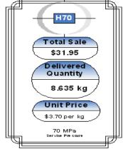
**Figure 1.** Examples of the product i dentity, measurement unit, unit price, and service pressure on the user's interface of a hydrogen Fuel Dispenser
