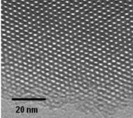
3 nm Silicate pores
