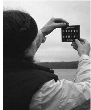
Volunteer using a color comparator, or colorimetric field kit (photo by K. Register).
