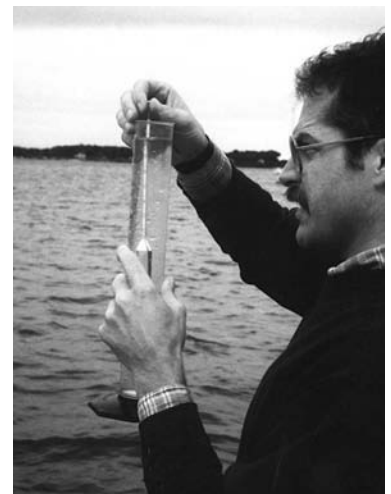
Using a hydrometer. (photo by P. Bergstrom).
