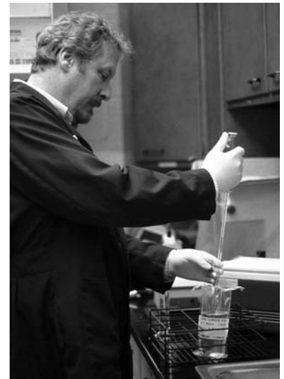
A measured amount of a water sample is being removed from a Whirl-pak bag prior to testing for the presence of bacteria. The sample has been kept cold since it was collected 3 hours before. Note that the volunteer is wearing gloves (photo by K. Register).
