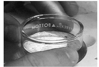
After incubation, any fecal coliform bacteria in the water sample will have grown into a colony (when using mFC medium or broth). These are called colony forming units (cfu) (photo by University of Maine Cooperative Extension).
