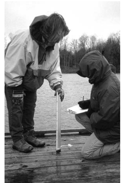
Using a transparency tube is an easy way to measure the water transparency. It is especially useful in water that is too shallow for a Secchi disk (photo by K. Register).
