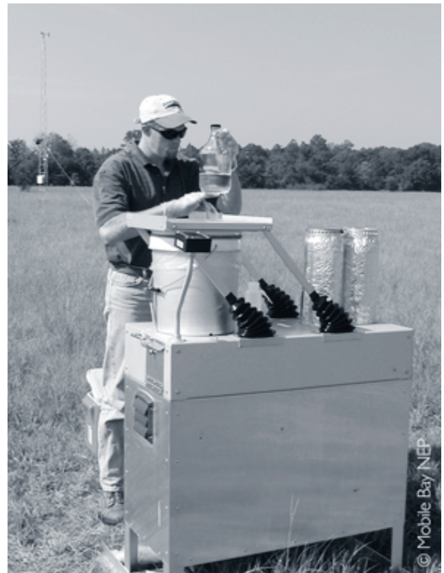
Atmospheric deposition is often monitored in NEP study areas because it can contribute to estuarine nitrogen loadings (Mobile Bay NEP).
