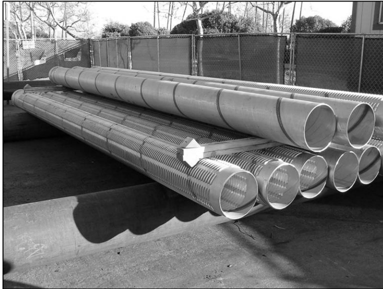
Photograph 4. Type 316L stainless steel 12 3 / 4 -in-OD louvered screen and casing delivered to the site (February 22, 2006).
