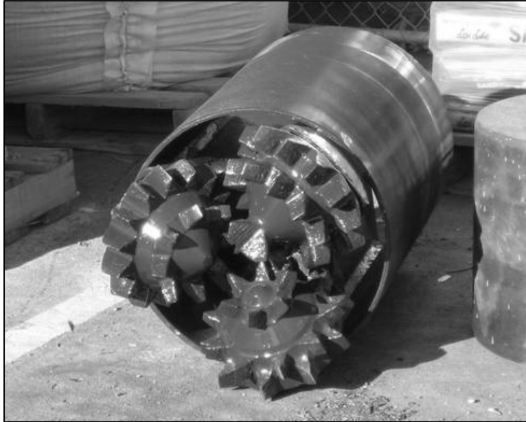
Photograph 17. 20-in. drill bit with integral stabilizer (February 9, 2006).
