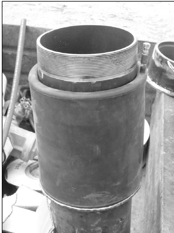
Photograph 13. Inflatable rubber packer used for isolating and testing the deep zone (May 3, 2006).
